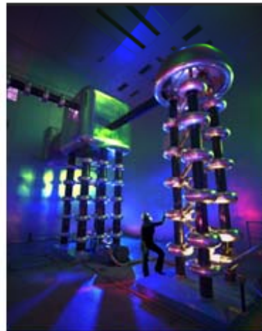
Cockroft-Walton accelerator: H + ions produced and accelerated up to 750 keV
