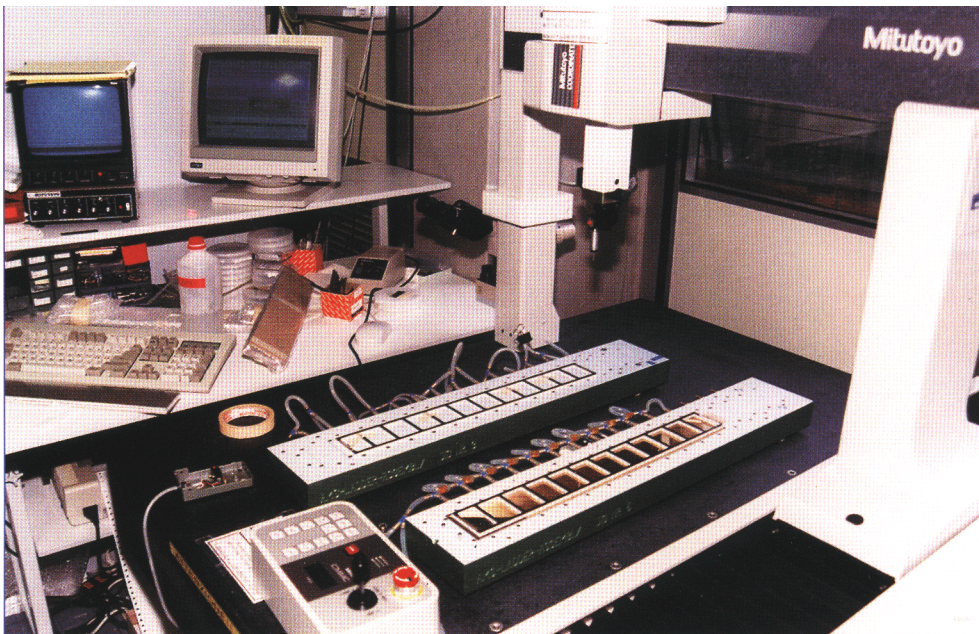
High precision tri-dimensional metrology machine used at the University of Perugia.
