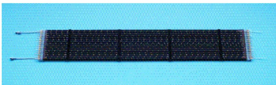
**Figure 45: TRD straw module as produced for the CERN 2001 testbeam.**
