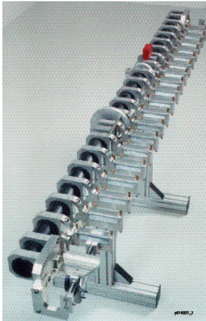
**Figure 49: Precision jig for the straw module assembly.**
