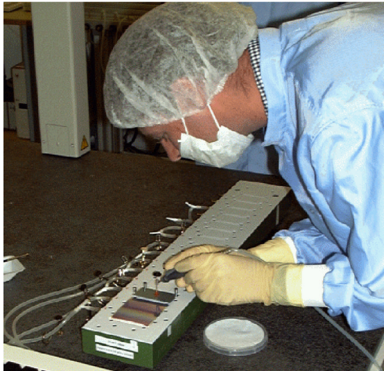
Figure 70 (left): Sensor positioning under metrology control. Figure 71 (right): wire bonding of sensors, on a silicon ladder of the AMS-02 production (Geneva University and CERN/ETHZ).
