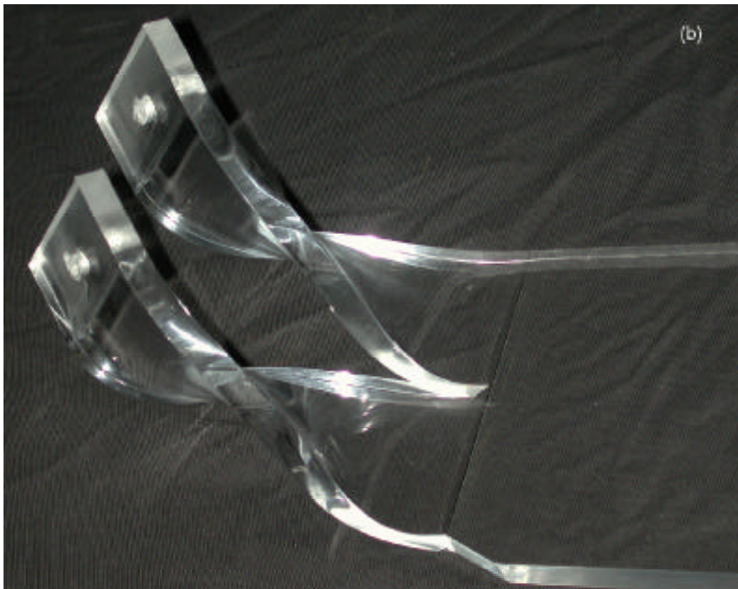
Figure 86: (a) General TOF counter design. The configuration of the light guides and the dimension of the clear plastic section are different for counters in different positions. (b) Photograph of sample light guide after tilting. The straight section on top of the guide has a hole to hold it during tilting and will be cut away before mounting
