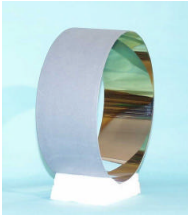
Figure 106: Cylindrical reflector model at scale 1:5.
