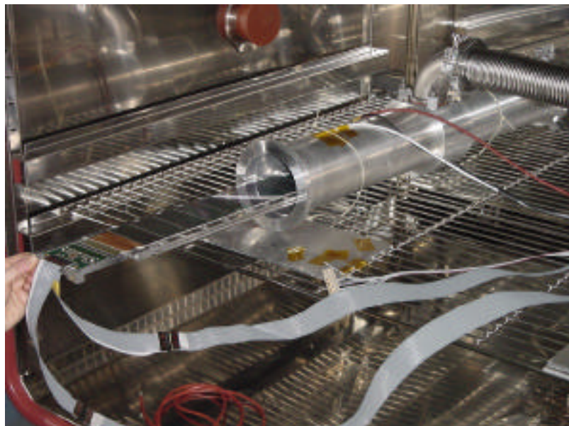
Figure 72: Thermovacuum test of an AMS-02 silicon ladder at the University of Perugia.
