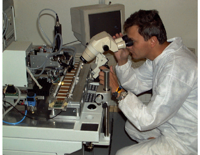
Figure 70 (left): Sensor positioning under metrology control. Figure 71 (right): wire bonding of sensors, on a silicon ladder of the AMS-02 production (Geneva University and CERN/ETHZ).
