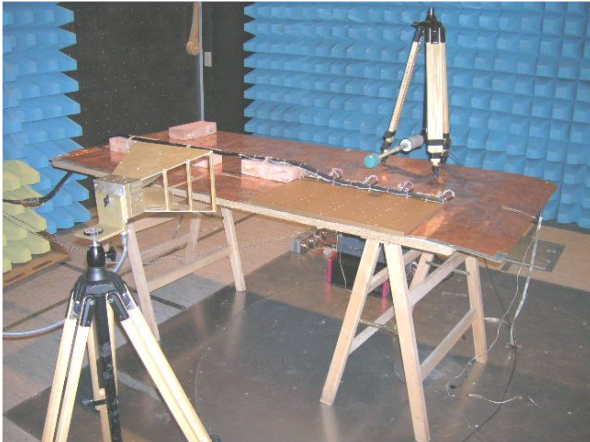
Fig. 9e: Radiated Susceptibility, Electric Field, 14 kHz ÷ 18 GHz (RS03) – part 5: 1 GHz ÷ 18 GHz.
