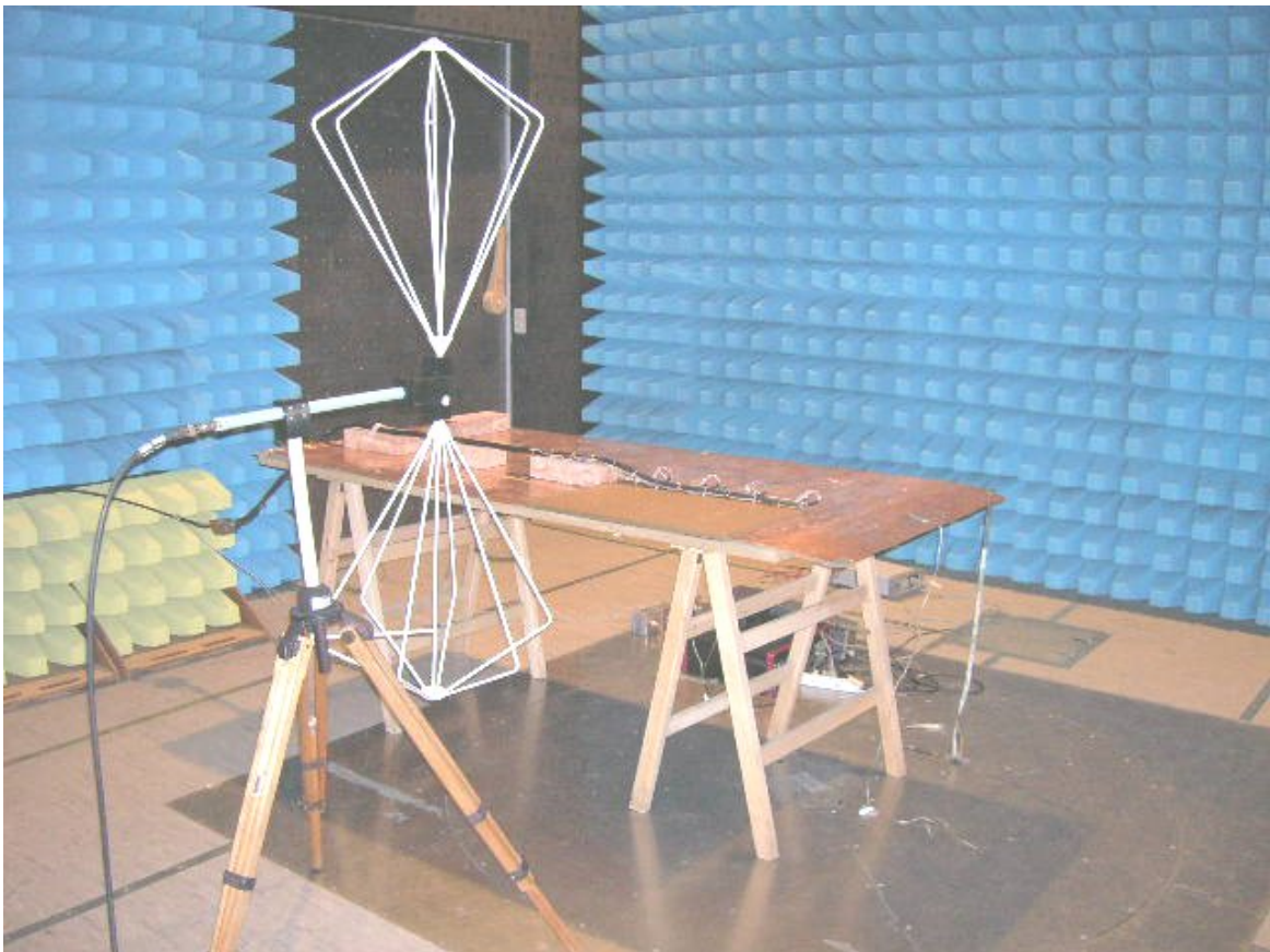
Fig. 7a: Radiated Emissions, Electric Field, 14 kHz ÷ 15,5 GHz (RE02) – part 1: 14 kHz ÷ 30 MHz.
