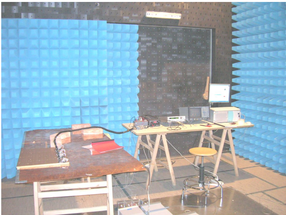
Fig. 6: Conducted Susceptibility, Spikes, DC Power Leads, (CS06).
