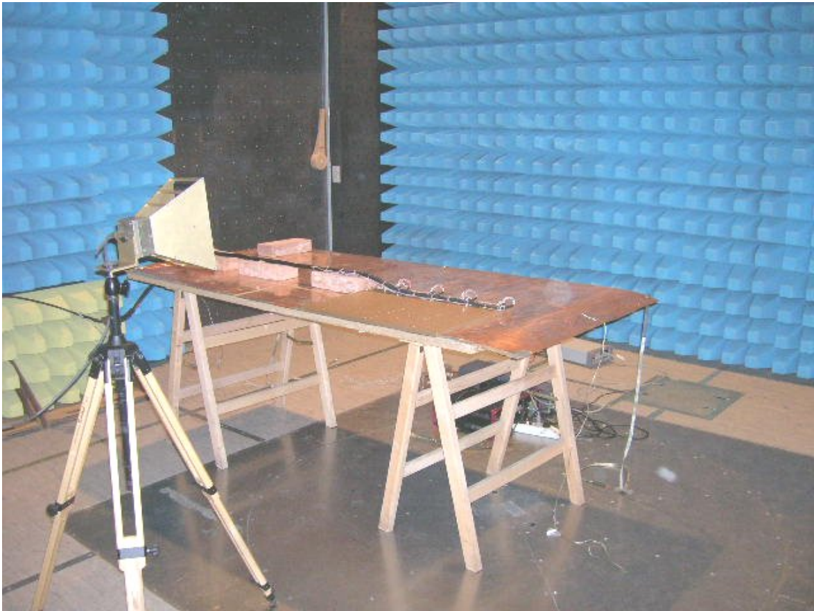
Fig. 7d: Radiated Emissions, Electric Field, 14 kHz ÷ 15,5 GHz (RE02) – part 4: 1 GHz ÷ 15,5 GHz.
