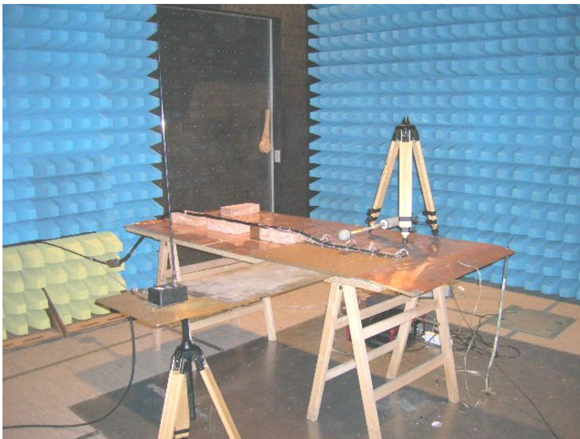
Fig. 9a: Radiated Susceptibility, Electric Field, 14 kHz ÷ 18 GHz (RS03) – part 1: 14 kHz ÷ 100 kHz.
