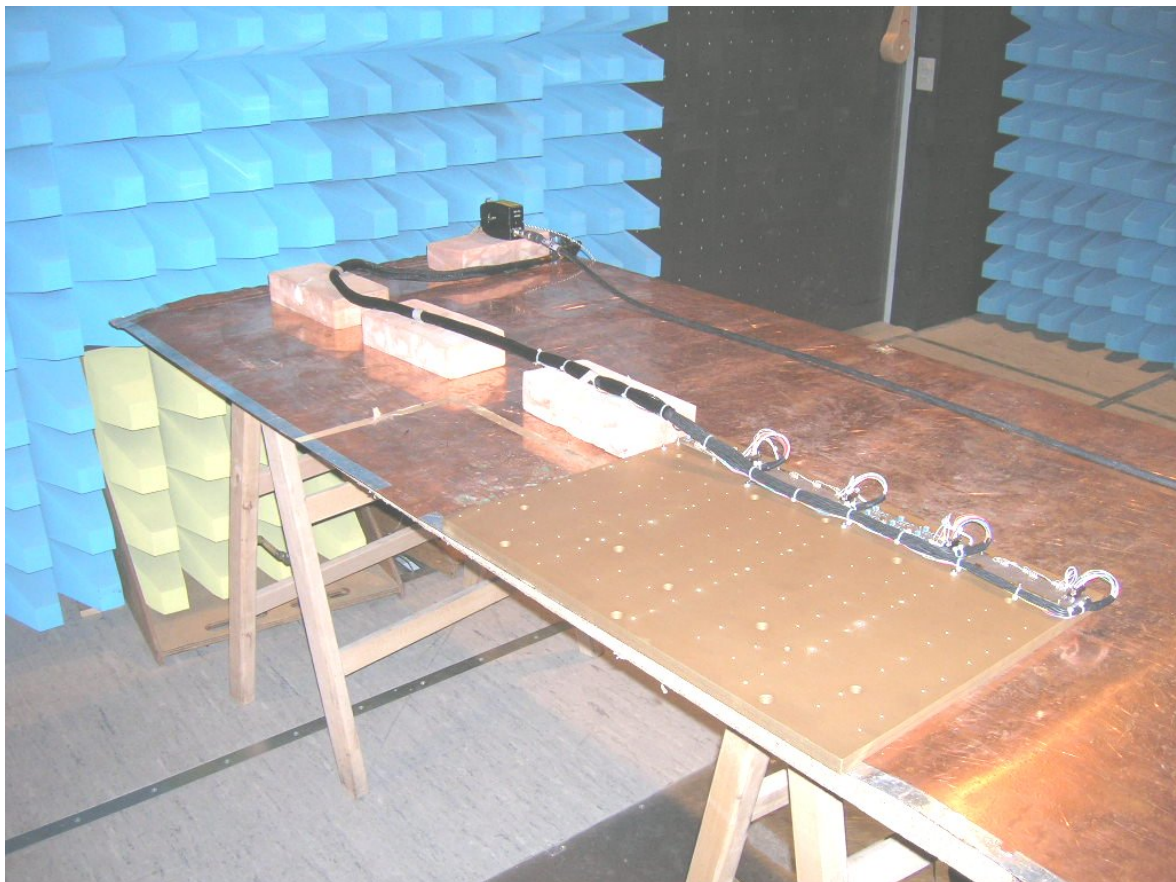
Fig. 2: Conducted Emissions, DC Power Leads, 15 kHz ÷ 50 MHz (CE03).
