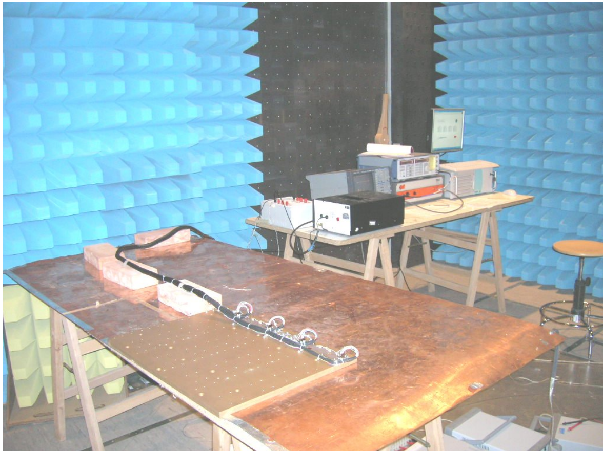
Fig. 5: Conducted Susceptibility, DC Power Leads, 50 kHz ÷ 50 MHz (CS02).
