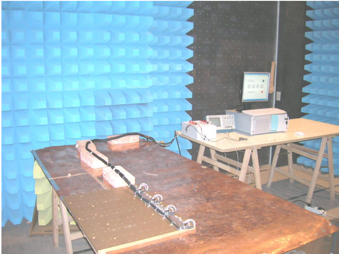
Fig. 3: Conducted Emissions, DC Power Leads, Switching Spikes, Time Domain (CE07).
