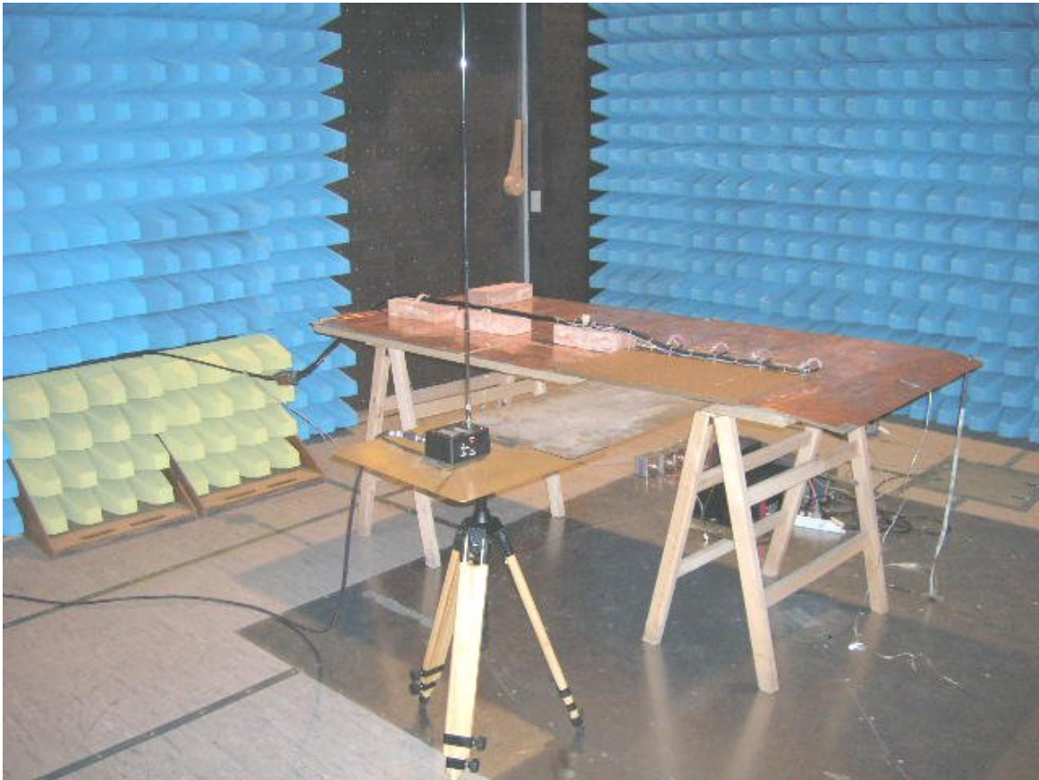
Fig. 7a: Radiated Emissions, Electric Field, 14 kHz ÷ 15,5 GHz (RE02) – part 1: 14 kHz ÷ 30 MHz.
