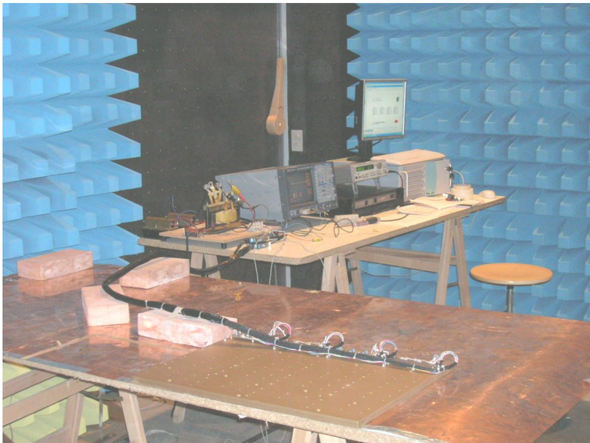
Fig. 4: Conducted Susceptibility, DC Power Leads, 30 Hz ÷ 50 kHz (CS01).
