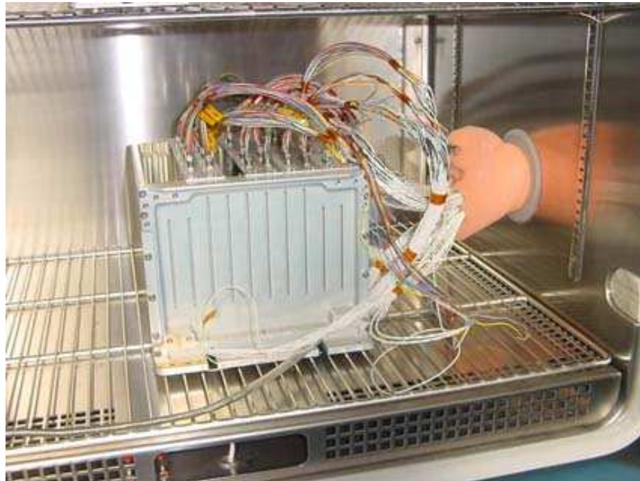
Figure 2 – UG crate FM placed inside the thermal chamber ready for the test.
