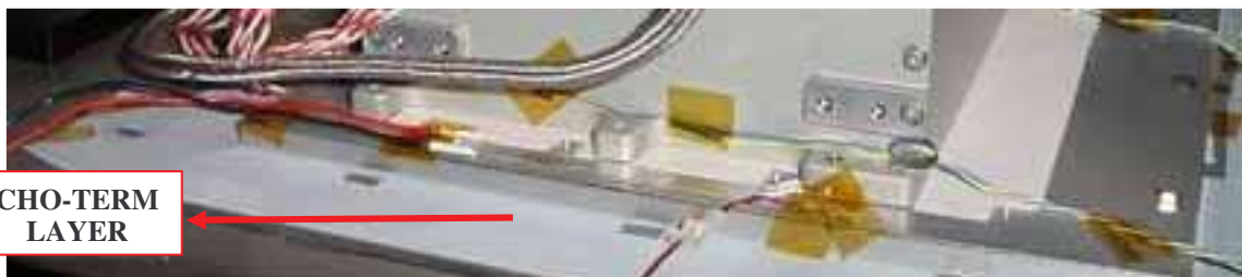
FIGURE 4 - DETAIL OF CHO-TERM LAYER PLACED BETWEEN THE AL FIXTURE AND THE COLD PLATE.
