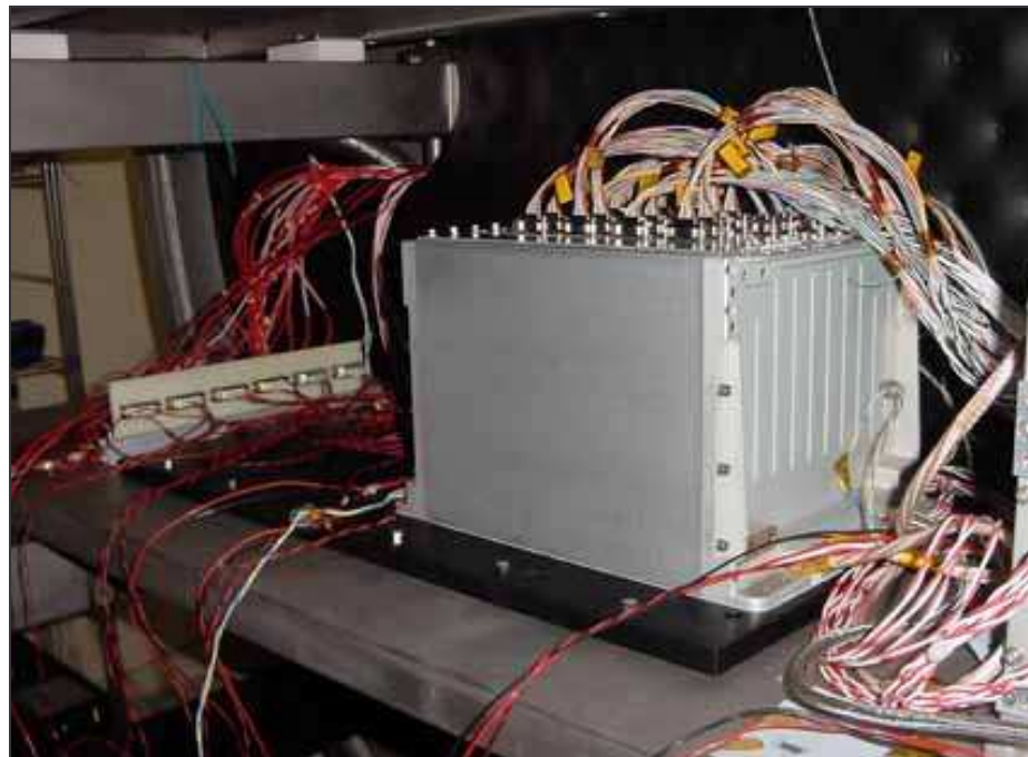
FIGURE 2 –UG CRATE INSIDE THE TVC, FIXED TO THE LOWER COLD PLATE.
