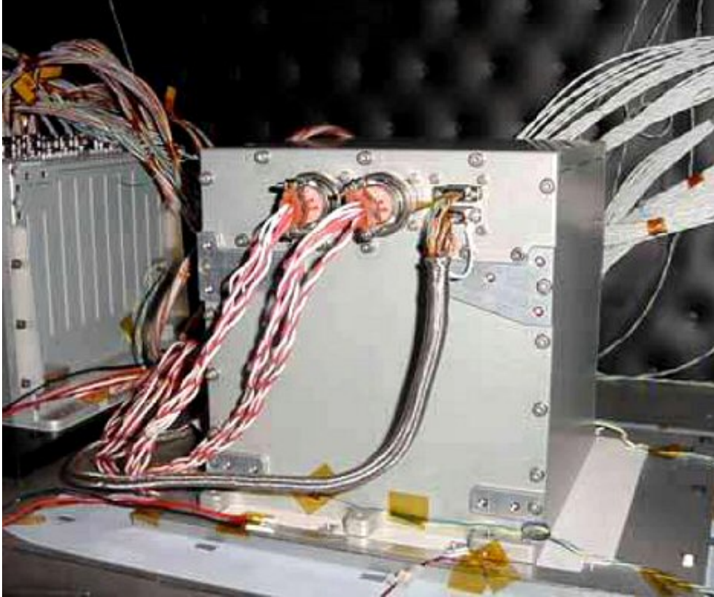
Figure 9: The UG electronics and the UGPD in the thermo-vacuum chamber.
