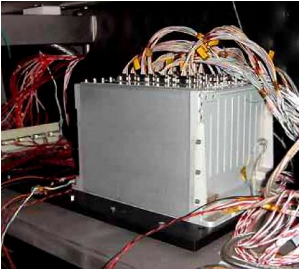
Figure 8: The UG electronics in the thermo-vacuum chamber.
