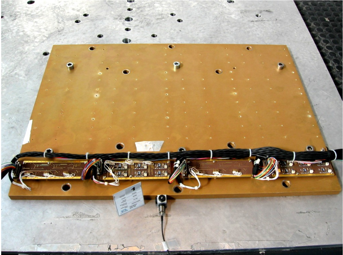
Figure 4. Control channel (CH1) in the Y-axis test setup.
