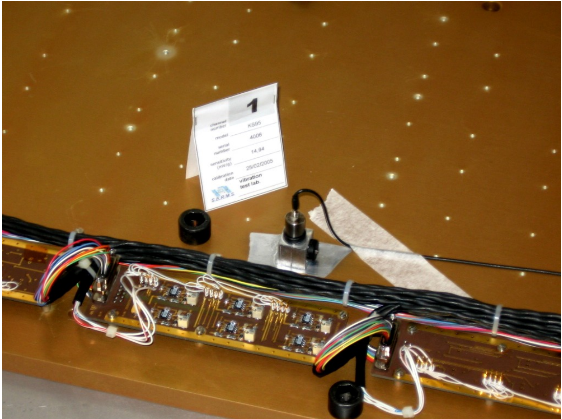
Figure 6. Control channel (CH1) in the Z-axis test setup.
