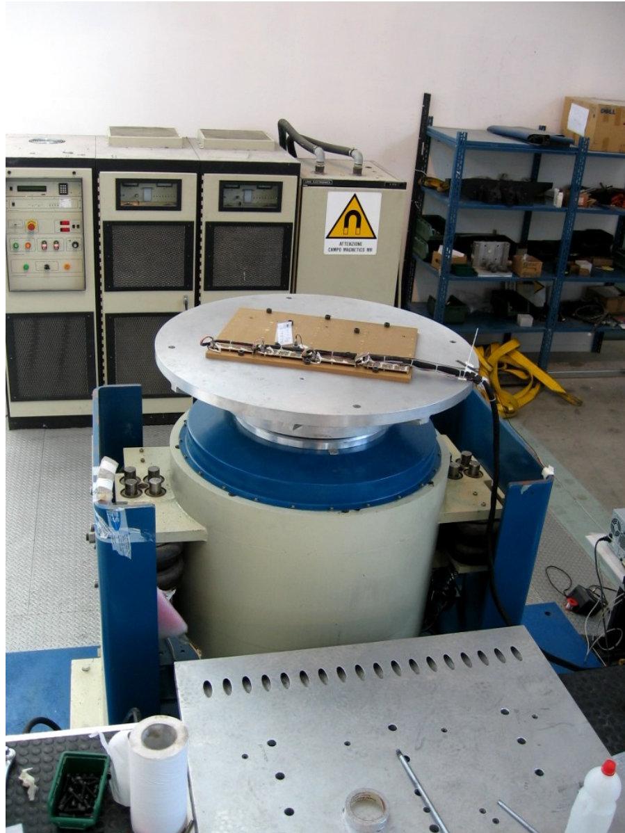
Figure 5. General view of the Z-axis test setup.
