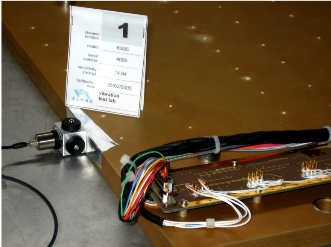
Figure 2. Control channel (CH1) in the X-axis test setup.
