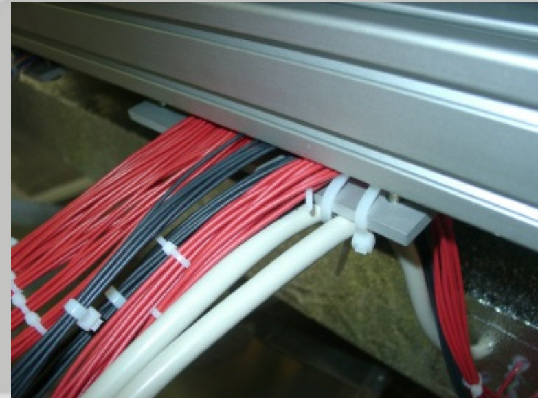
TRD-HV Cables to U-crate under right Rosengitter bar ToF cables to S-crate
