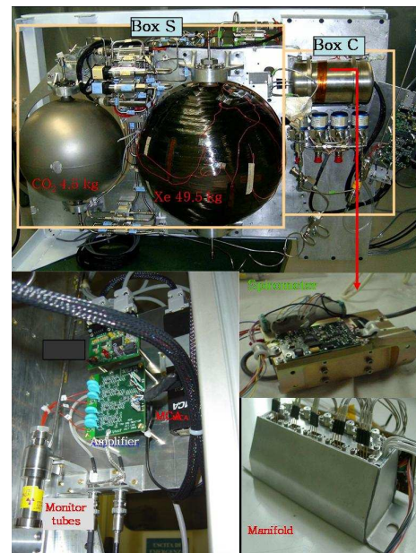
Fig. 5. TRD gas system with the monitor tubes, the spirometer and a manifold.
