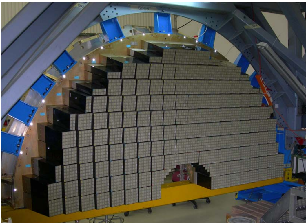
Figure 4.7: An endcap Dee, fully equipped with supercrystals.
