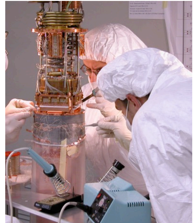
... the connection of the tower to the MC of dilution refrigerator.
