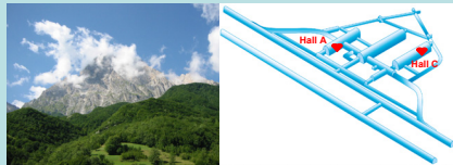
Figure 3. The CUORE experiment will be housed underground at the Gran Sasso National Laboratories in Italy. The underground facility consists of 3 experimental halls. CUORE will operate in Hall A, next to Cuoricino. There is also an R&D cryostat located in Hall C.
