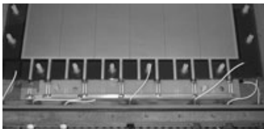
Figure 5.2: The resistor chain used to supply the different sectors.
