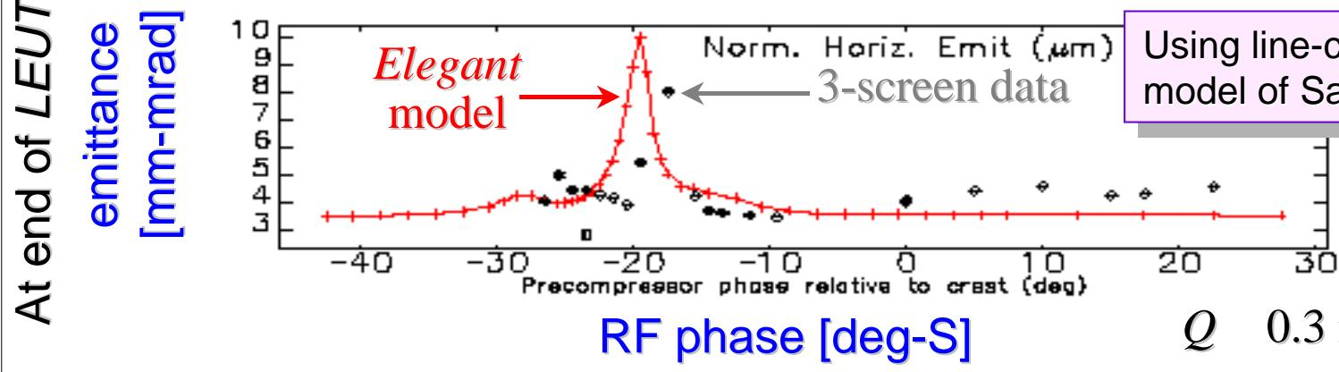
Using line-charge CSR model of Saldin, et. al.
