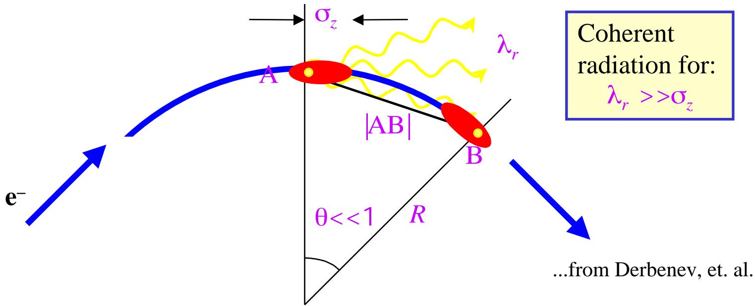
Free space radiation from bunch tail at point **A** overtakes bunch head, a distance  $s$  ahead of the source, at the point **B** which satisfies...
