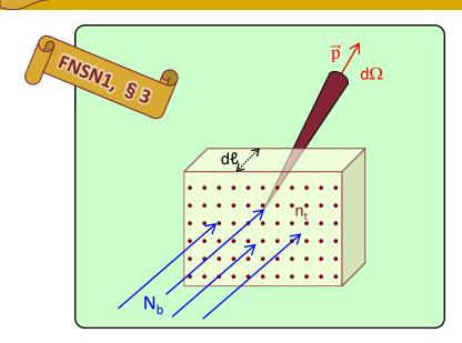
A beam of  $N_b$  particles is sent against a thin layer of thickness  $d\ell$ , containing  $N_t$  scattering centers in a volume  $\Phi$  ("target", density  $n_t = dN_t/d\Phi$ ).
