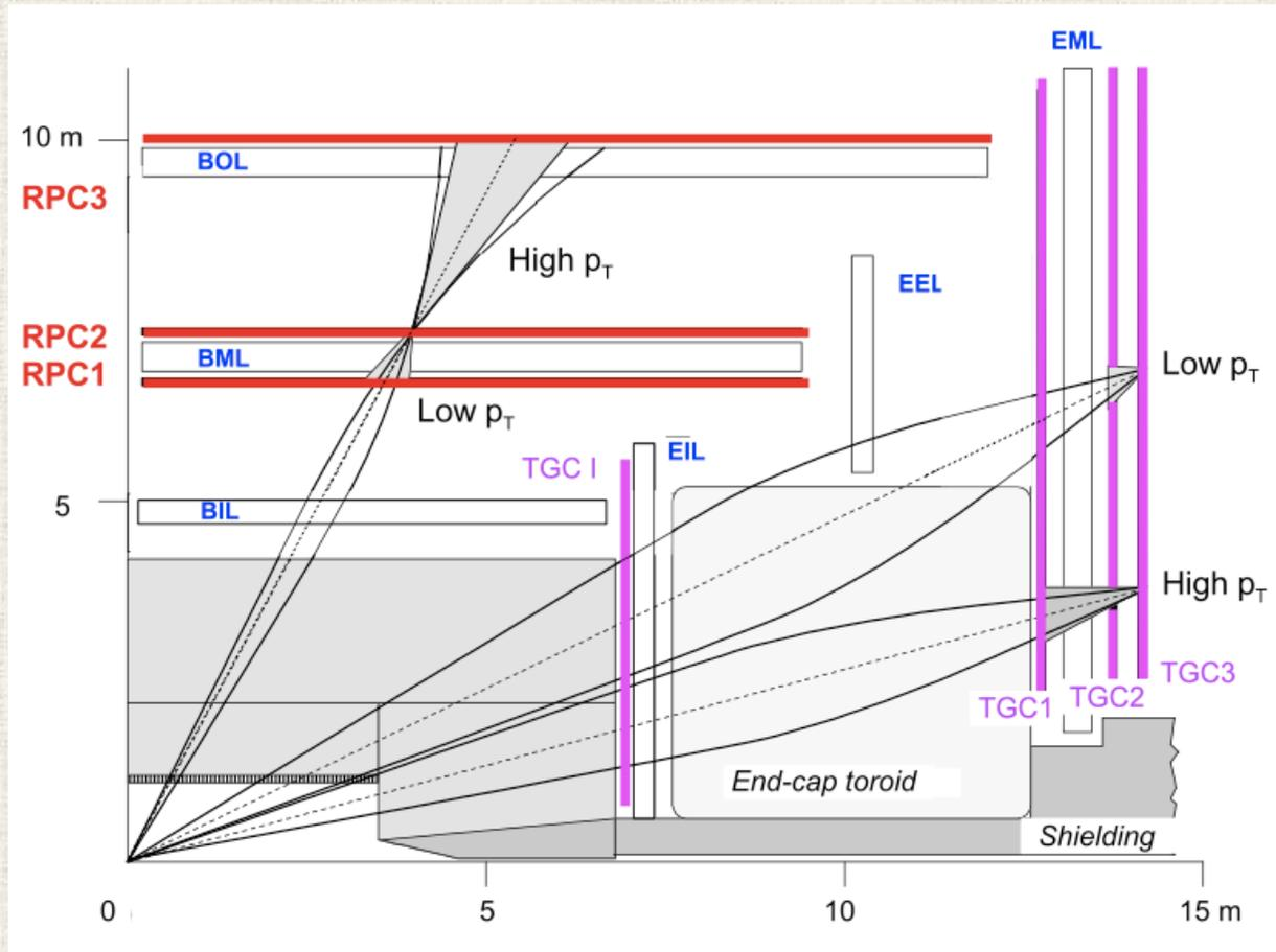
**Level-1:** fully hardware trigger, simply based on RPC or TGC coincidences, with up to 6  $p_T$  thresholds with full  $\eta$  coverage;
