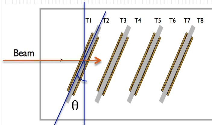
8 chambers  $10 \times 10 \text{ cm}^2$  x-y view  $400 \mu\text{m}$  pitch
