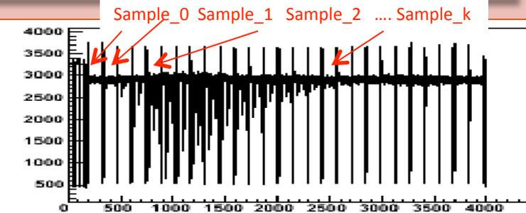
Strip waveform as a function of time (1 sample = 25 ns)
