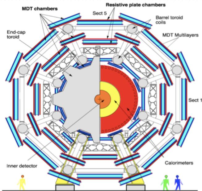
“Small” wheel: region with highest rate up to  $10 \div 15 \text{ kHz/cm}^2 @ 5 \times 10^{34} \text{ cm}^{-2} \text{ s}^{-1}$
