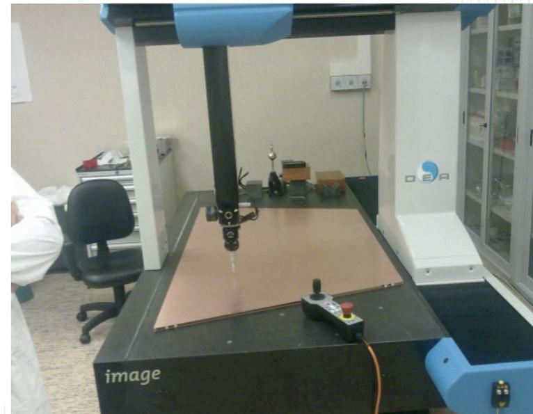
RMS below  $20 \div 30 \mu\text{m}$  obtained in prototype panels of  $1 \div 2 \text{ m}^2$  size
