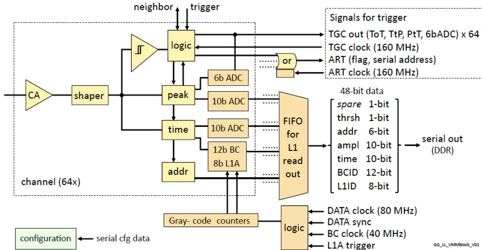
Figure 12.3: Block diagram of the VMM ASIC
