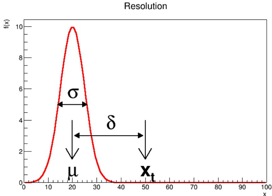
FIGURE 3. Example of a gaussian response function (red) with  $\mu$  and  $\sigma$  and comparison with the true value  $x_t$ .  $\delta$  is the systematic error. The outcome of the measurement  $x_m$  is distributed according to the apparatus response function. The length of the double arrow indicating the  $\sigma$  is actually the function FWHM (full width half maximum) that in case of a gaussian function is  $\text{FWHM}=2.36 \times \sigma$ .
