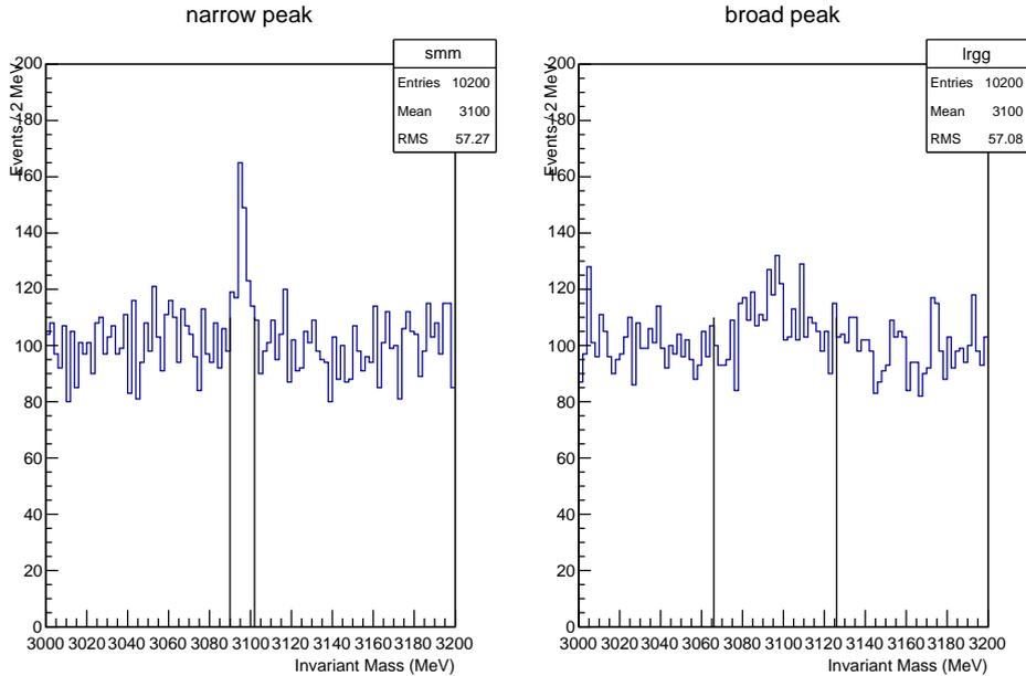
FIGURE 8. Simulation of  $S = 200 J/\psi$  events superimposed to a flat background of 10000 distributed on a range of 200 MeV ( $b=50 \text{ MeV}-1$ ).  $\sigma_M = 2 \text{ MeV}$  (left) and  $\sigma_M = 10 \text{ MeV}$  (right). The limits of  $\pm 3\sigma_M$  intervals around the expected position of the peak are shown. Outside these limits are the sidebands.
