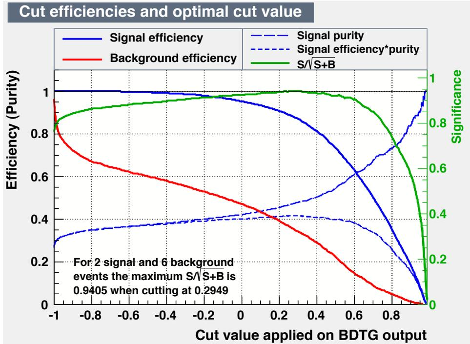
FIGURE 7. Several quantities are shown as a function of the possible value of  $t_{cut}$ , the cut on the BDT variable. Blue and red curves show respectively the signal and background efficiency while the green curve is the score function that, in this case, has a maximum around  $t_{cut} = 0.25$  although with a very low significance (below 1). (taken from A.Calandri thesis, Sapienza University, A.A. 2011-2012)
