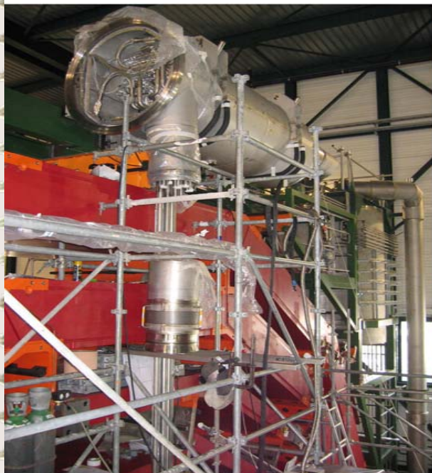
The cryogenic chimney links the cold mass to the phase separator cryostat by SDMS (F)
