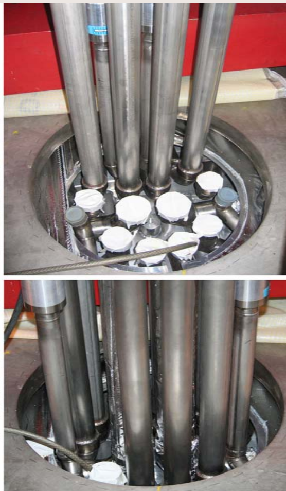
The cryogenic chimney links the cold mass to the phase separator cryostat by SDMS (F)
