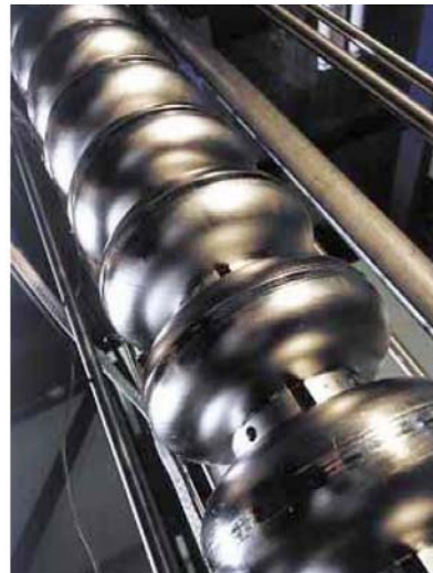
Superconducting, L-band standing wave cavity
