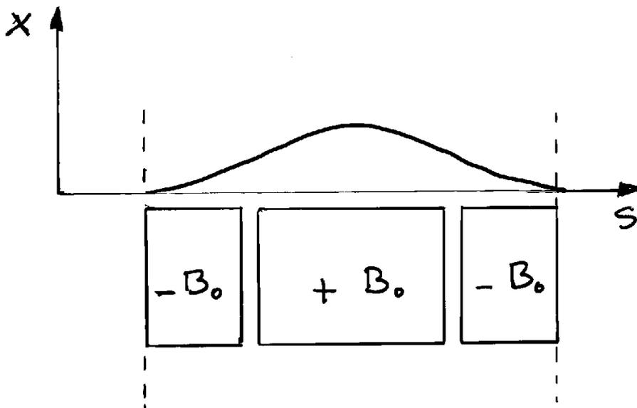
**Wigglers are also used in synchrotron light sources to increase the critical frequency and the emitted power with respect to that of the bending magnets.**
