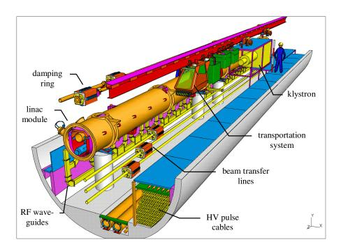
FIGURE 3.3. Sketch of the 5 m diameter TESLA linac tunnel.
