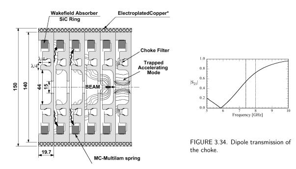
FIGURE 3.33. Cut-away view of the C-band choke-mode structure.
