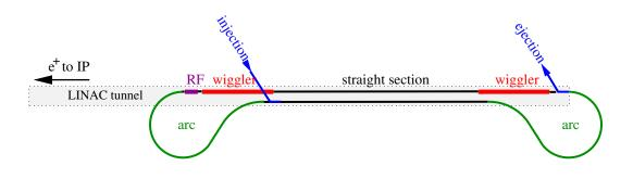
FIGURE 3.13. Conceptual layout of the positron damping ring. The electron ring is similar with the exception that the injection point is located close to the indicated ejection position at the beginning of the linac.
