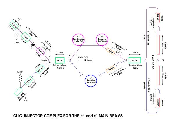
FIGURE 3.58. CLIC injector complex for the  $e^+$  and  $e^-$  main beams.
