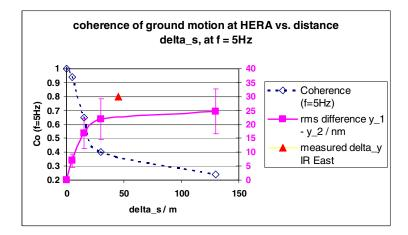
FIGURE 3.19. Relative rms vibration amplitude ( $f \ge 5$  Hz) in the HERA tunnel as a function of distance between the points where the seismometers were placed (squares, right hand scale) and the measured coherence (diamonds, left hand scale). These data were taken in 1995. A more recent (2000) result for the difference amplitude across the interaction region East is also shown (triangle).
