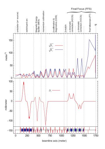
FIGURE 3.15. Optics functions for the TESLA BDS  $(e^{-})$ .
