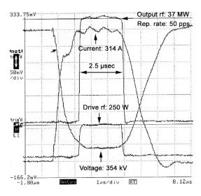
FIGURE 3.29. Output waveform of C-band PPM klystron.
