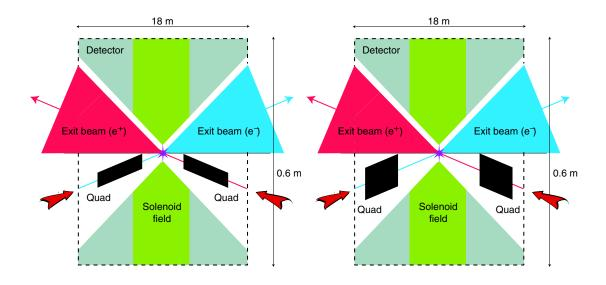
FIGURE 3.67. Top view of the CLIC IP region with the detector, the colliding beams, and the final quadrupoles for the base-line (left) and the compact final-focus optics (right) at 3 TeV. Scales are indicated. The transverse size of the detector is about 17 m.
