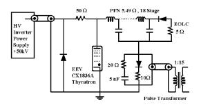
FIGURE 3.23. Schematic diagram of the C-band modulator circuit.
