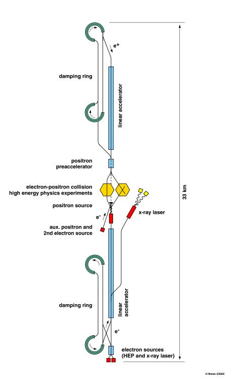
FIGURE 3.2. Sketch of the overall layout of TESLA.
