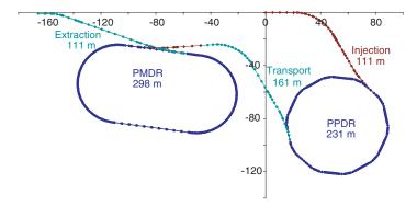
FIGURE 3.47. Schematic of NLC positron damping ring complex.
