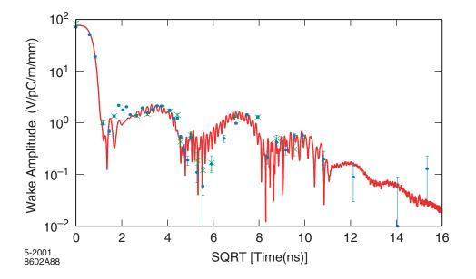
FIGURE 3.45. Comparison of measured and predicted wakefield for the RDDS1 structure.
