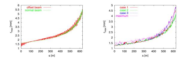
FIGURE 3.78. Left: The  $3\sigma$ -envelope of a beam with initial offsets of  $\Delta x = \sigma_x$  and  $\Delta y = \sigma_y$ . For comparison the  $4\sigma$ -envelope of a beam with no offset is also shown. Right: the  $3\sigma$ -envelopes in a decelerator after beam-based alignment. Three examples are shown together with the envelope that contains all of 100 simulated cases.
