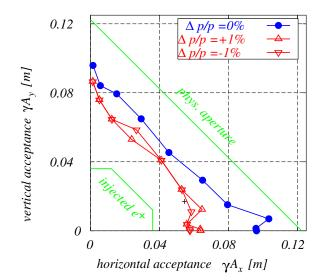
FIGURE 3.14. Dynamic acceptance of the damping ring. The simulations include quadrupole and sextupole alignment errors which result in an average emittance coupling of 1%, and the real physical aperture as the maximum amplitude limit. The phase space volume of the incoming beam as defined by acceptance of the positron pre-accelerator is also shown.
