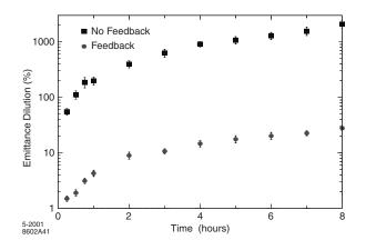
FIGURE 3.55. Emittance dilution (%) in the NLC main linacs due to diffusive ground motion, assuming an ATL coefficient comparable to that measured at SLAC. A case with no linac feedbacks (squares) and a case with the proposed NLC steering feedback architecture (circles) are both considered.
