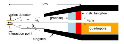
FIGURE 3.68. View from above on the adopted mask design. The sketch is stretched in the vertical direction. Care has to be taken that no particles are backscattered through the hole in the mask.
