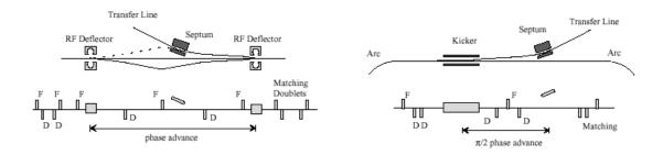
FIGURE 3.76. Schematic layout of the injection insertion with rf deflectors (left) and of the extraction insertion (right). At injection, the circulating bunches will travel on the central or inner orbit, while the injected bunches are kicked by the  $2^{nd}$  deflector onto the equilibrium orbit. The train of combined bunches is ejected before the next pulse reaches the deflecting phase represented by the dotted line trajectory (intercepting the septum).
