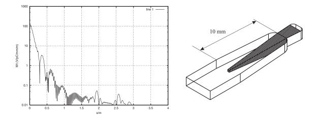
FIGURE 3.65. Left: Transverse wake of the TDS with the 10 mm load, as computed by the double-band circuit model (n.b. the computation has been made for a 15 GHz structure). Right: Detail of the TDS load. The load is 2 mm wide at its base and 0.2 mm<sup>2</sup> at the tip.
