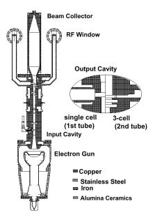
FIGURE 3.25. Cross-sectional view of the E3746 C-band klystron.
