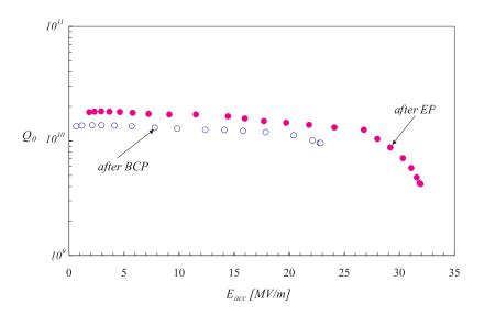
FIGURE 3.7. Excitation curve of a TESLA 9-cell cavity after buffered chemical polishing (BCP) and electropolishing (EP), but before application of the baking procedure.
