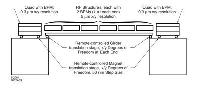
FIGURE 3.53. Beam-based alignment hardware in the NLC main linac.
