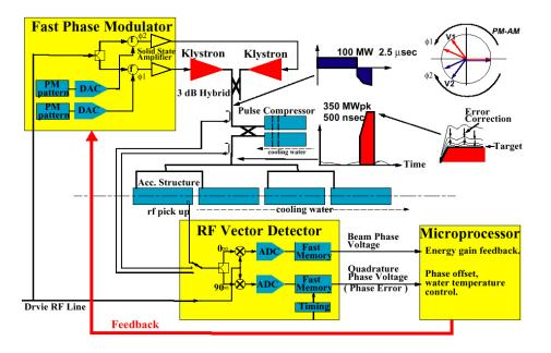
FIGURE 3.31. Schematic diagram of the phase modulation system.
