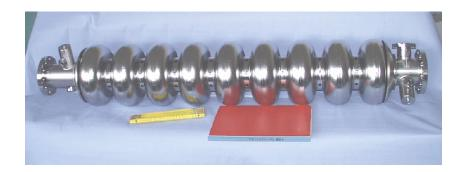
FIGURE 3.1. The 9-cell niobium cavity for TESLA.
