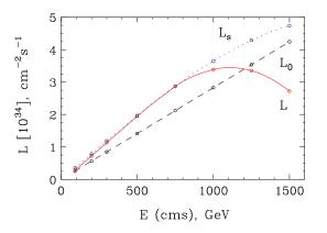
FIGURE 3.50. Energy reach of the NLC final focus where  $L_0$  is the luminosity without the pinch enhancement, L is the nominal luminosity, and  $L_s$  is the luminosity after scaling the bending magnets. By scaling the bending magnets in a manner to maintain the IP position the present system can accommodate beam energies well above 1500 GeV.
