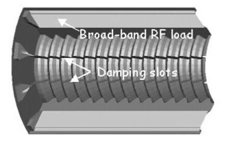
FIGURE 3.79. A quarter geometry of the C-PETS with 12 damping slots and SiC loads.
