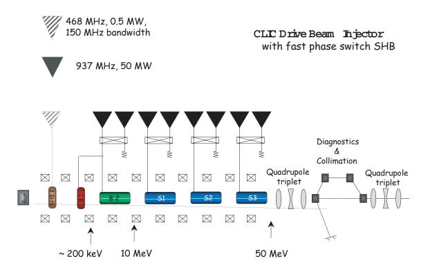
FIGURE 3.70. Layout of the CLIC Drive Beam Injector.
