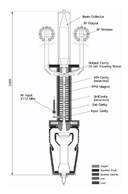
FIGURE 3.28. Cut-away view of the first C-band PPM klystron, TOSHIBA-E3747.
