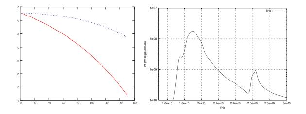
FIGURE 3.64. Left: Accelerating gradient in MV/m as a function of cell number. The solid line is with beam and the dotted one without. Right: Transverse wake spectrum in V/Hz/pC/mm/m between 16 and 30 GHz.
