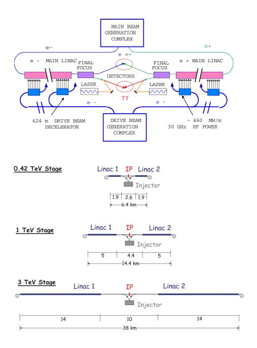
FIGURE 3.57. The top shows the overall layout of the CLIC complex and the bottom shows the tunnel lengths (km) for the linacs and the BDS (base-line design) on each side of the IP, at various cm energies.
