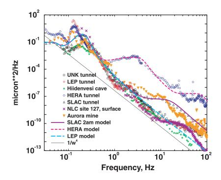
FIGURE 3.52. Power spectrum of ground motion, in units of  $\mu m^2/Hz$ , from several accelerator tunnels and a cave. The strong peak at 0.15 Hz in all spectra is from ocean waves. The shoulder at 4 Hz in the HERA data is most likely due to "cultural noise," vibration sources within the accelerator complex and from the surrounding urban area.
