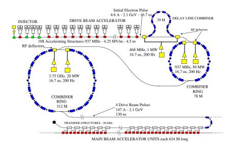
FIGURE 3.74. Drive-beam klystron-modulators for one generation complex.
