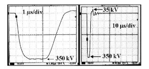
FIGURE 3.24. Output waveform of the modulator.
