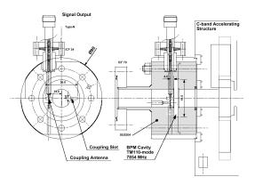
FIGURE 3.37. RF BPM with common-modeless design.
