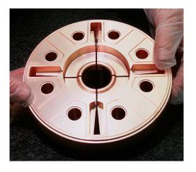
FIGURE 3.73. Left: Conceptual view of the SICA accelerator structure. Right: Machined disc of the 3 GHz version of the SICA structure.
