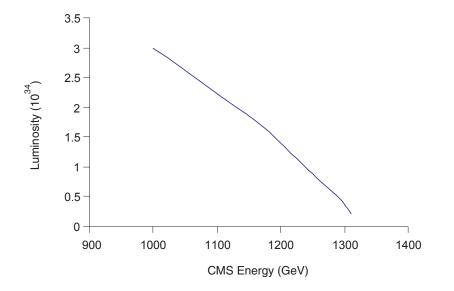
FIGURE 3.39. Energy versus luminosity for Stage II NLC rf system.
