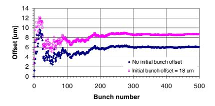
FIGURE 3.11. Orbit offsets in  $\mu$ m of the first 500 bunches at the end of the linac. The lower curve shows the effects of cavity misalignments only ( $\Delta y_c = 0.5 \text{ mm rms}$ , one seed). The upper curve shows the effects of the same misalignments, but with an additional one  $\sigma_y$  injection error of the beam (coherent betatron oscillation).
