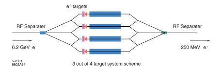
FIGURE 3.46. Schematic of the conventional  $e^+$  production system.
