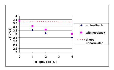
FIGURE 3.20. Luminosity as a function of correlated emittance growth obtained from beam-beam simulations (see text). The diamonds are the results without feedback, the squares with IP steering feedback "on." The dashed line denotes the expected luminosity if the emittance growth was uncorrelated.
