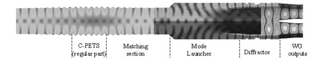
FIGURE 3.80. The electric field pattern of the rf power extractor for the C-PETS.
