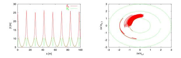
FIGURE 3.72. Left: The beta functions in the drive beam accelerator. Right: The final offset of a beam entering the structure with an offset of one rms bunch size  $\sigma$ . The value is normalized to the final beam size.
