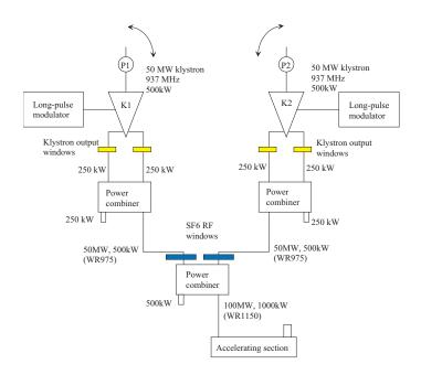
FIGURE 3.75. 50 MW MBK rf module layout.
