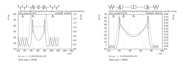
FIGURE 3.60. Left: Optical functions in the first chicane. Right: in the second chicane.
