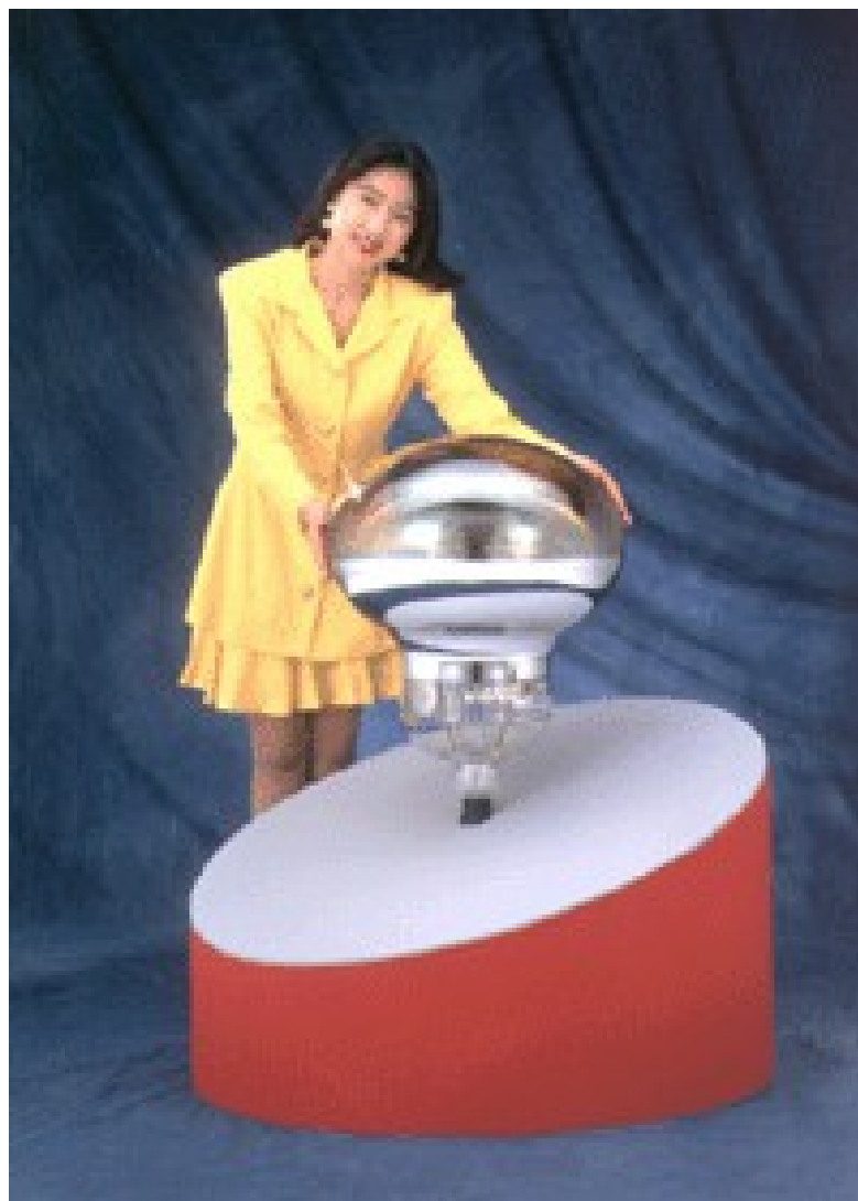
20" PMT by Hamamatsu Photonics
