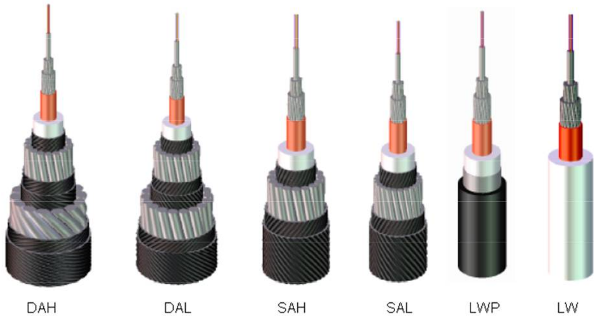
Figure 7-16: Different armoring on submarine cable.
