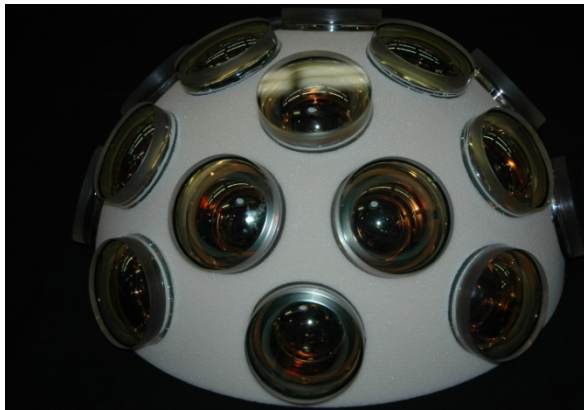
Figure 7-4: 20 3" photomultipliers in their Styrofoam support
