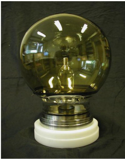
Figure 7-8: Spherical geometry X-HPD (8" prototype): (CERN-Photonis collaboration).
