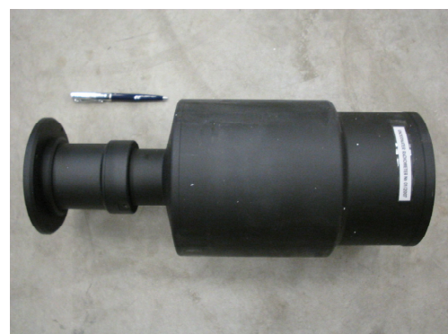
Figure 6-14: Probe for 40 K monitoring
