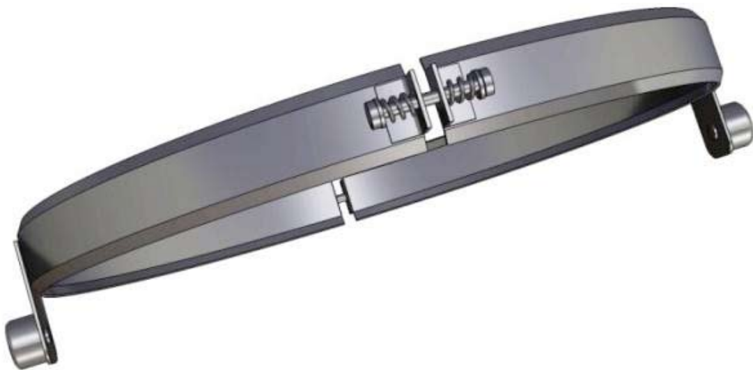
Figure 3-30: The spring loaded titanium connection ring
