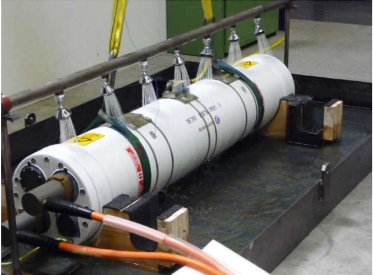
Figure 3-42: The Medium Voltage Converter.
