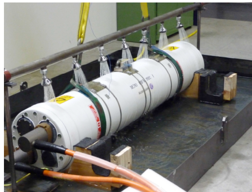
Fig. 9 – The Medium Voltage Converter complete assembly
