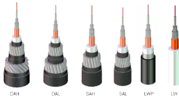
Fig. 4.2 – Examples of different armouring on submarine cables.
