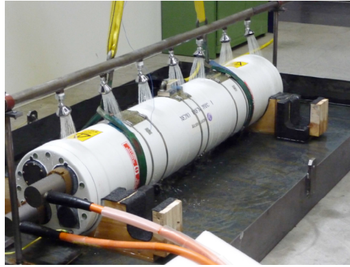
Fig. 2.33 – The Medium Voltage Converter complete assembly
