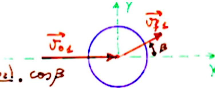
$$\begin{cases} V_{f1x}^* = \epsilon \frac{m_2 (V_{01} - V_{02})}{m_1 + m_2} \cos \beta \\ V_{f1y}^* = \epsilon \frac{m_2 (V_{01} - V_{02})}{m_1 + m_2} \sin \beta \end{cases}$$
