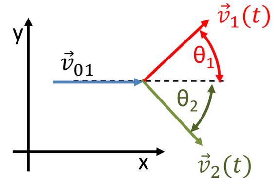
$$v_{1,x}(t) = \frac{v_{0,1}(m_1 + m_2 \cos 2\alpha)}{m_1 + m_2} ; \quad v_{1,y}(t) = \frac{m_2 v_{0,1} \sin 2\alpha}{m_1 + m_2}$$
