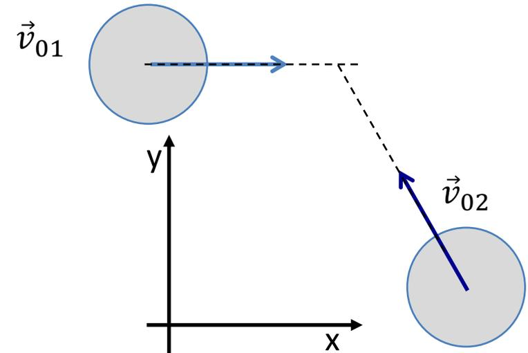
$$\vec{v}'_{01} = \vec{v}_{01} - \vec{v}_{CM} = \frac{\vec{v}_{01}(m_1+m_2) - m_1\vec{v}_{01} - m_2\vec{v}_{02}}{m_1+m_2} = \frac{\vec{v}_{01}m_2 - m_2\vec{v}_{02}}{m_1+m_2} = \frac{m_2}{m_1+m_2} (\vec{v}_{01} - \vec{v}_{02})$$
