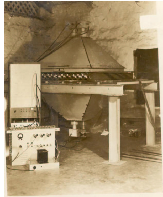
The scintillator-lead-GM counter telescope used at great depths in KGF mines. A coincidence of pulses from PMTs viewing the two scintillators and the sandwiched GM counter array provided the signal with negligible background.
