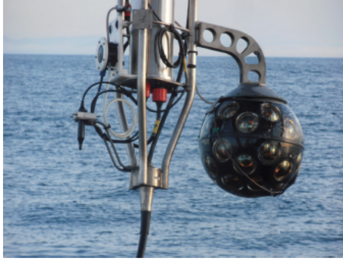
Figure 6.3. A KM3NeT Digital Optical Module: it contains 31 3-inch PMTs, pointing from vertically downwards to 45° upwards.
