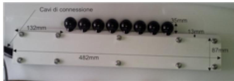
**Figure 3.1.** Acoustic source consisting of eight transducers.
