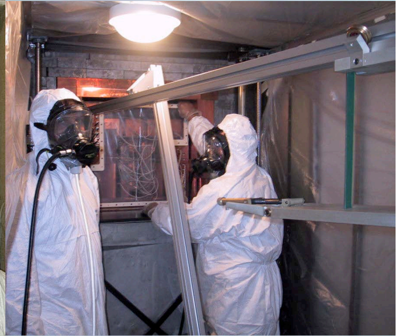
Dismounting the ~100kg NaI(Tl) set-up in August 2002 in HP N 2 atmosphere
