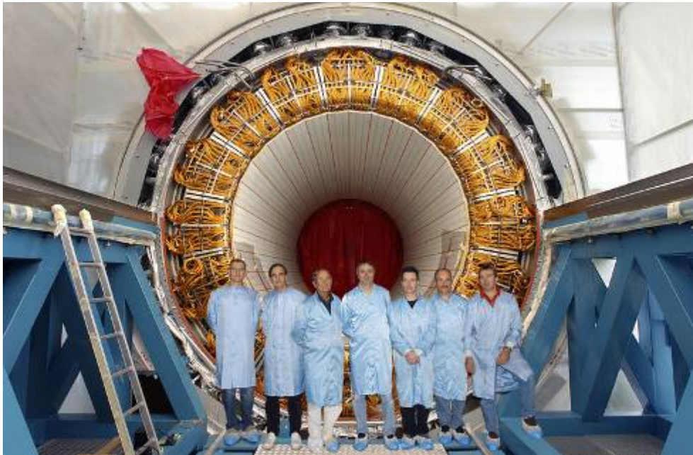
LAr barrel EM calorimeter after insertion into the cryostat
