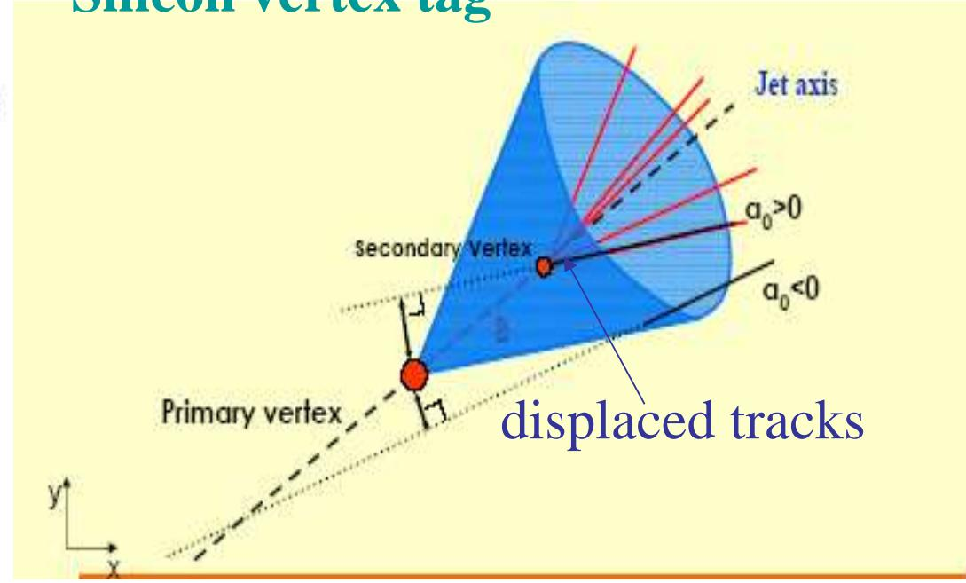
B mesons travel  $\sim 3\text{mm}$  before decaying – search for secondary vertex
