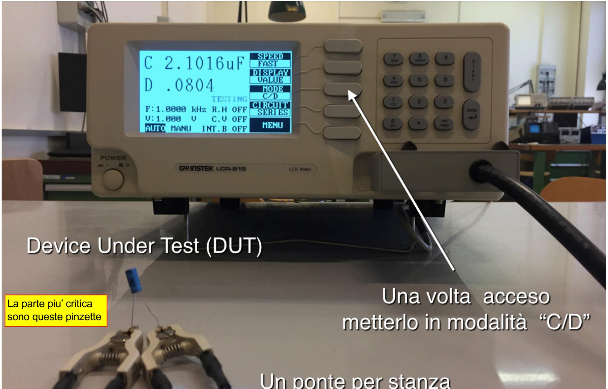
Device Under Test (DUT)
