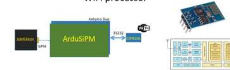
The ArduSiPM sends data over rs232, the Wifi Processor elaborate the data and send them using the MQTT protocol to the server. We use as network processor the Espressif ESP8266 a low-cost Wi-Fi chip with full TCP/IP stack and a 32-bit RISC CPU running at 80 MHz. The ESP8266 can be used to send and configure MQTT packets, NTP request and configure ArduSiPM device.
