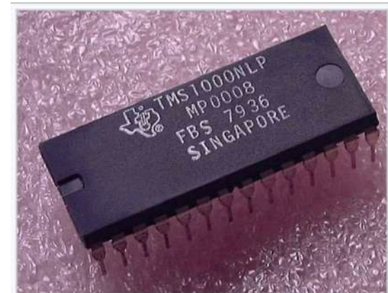
A TMS1000 "computer on a chip".
