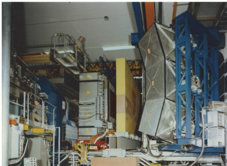
Fig. 4.3. Partial view of Axial Field Spectrometer at I8. The vertical uranium/scintillator hadron calorimeter (just left of centre) is retracted to give access to the cylindrical central drift chamber. The yellow iron structure served as a filter to identify muons, with MWPCs and the array of Cherenkov counters to the right.
