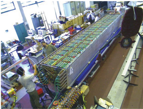
Fig. 4.20. One of the 18 modules of the ALICE TRD during final tests prior to installation. Six radiator-detector layers are contained in such a module. The last layer seen in the photo shows the signal and real-time trigger electronics, directly behind the X-ray detector. The radiator (insert) is made for technical reasons from mats of polypropylene fibres. (Source: University of Heidelberg).
