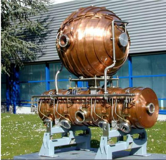
128 five-cell copper cavities, powered by 16 klystrons of 1 MW (maximum value, mean value delivered was 0.6 MW).
