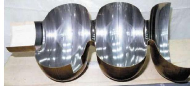
A superconducting cavity, cut in two. One can see the inner layer of sputtered niobium.
