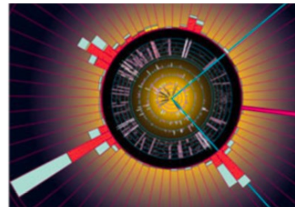
D0: two muons (in blue, one inside a jet), 4 jets and the neutrino (pink) identified as missing p_T
