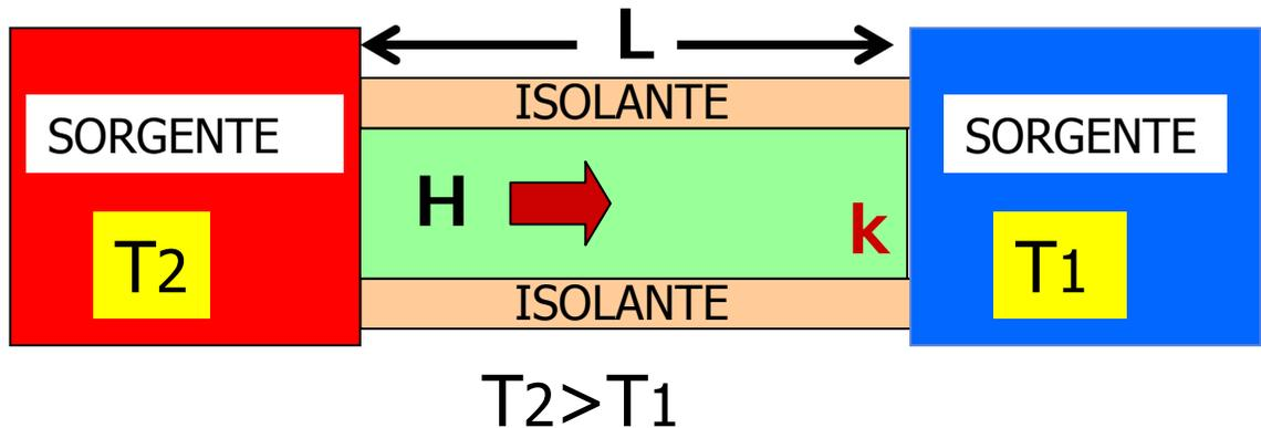
$$T_2 - T_1 = -\Delta T \quad ; \quad L = \Delta x \quad \Rightarrow \quad H = \frac{dQ}{dt} = -k \cdot A \frac{\Delta T}{\Delta x}$$
