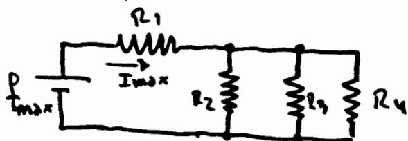
$$R_1 = 5\Omega ; R_2 = 30\Omega$$
