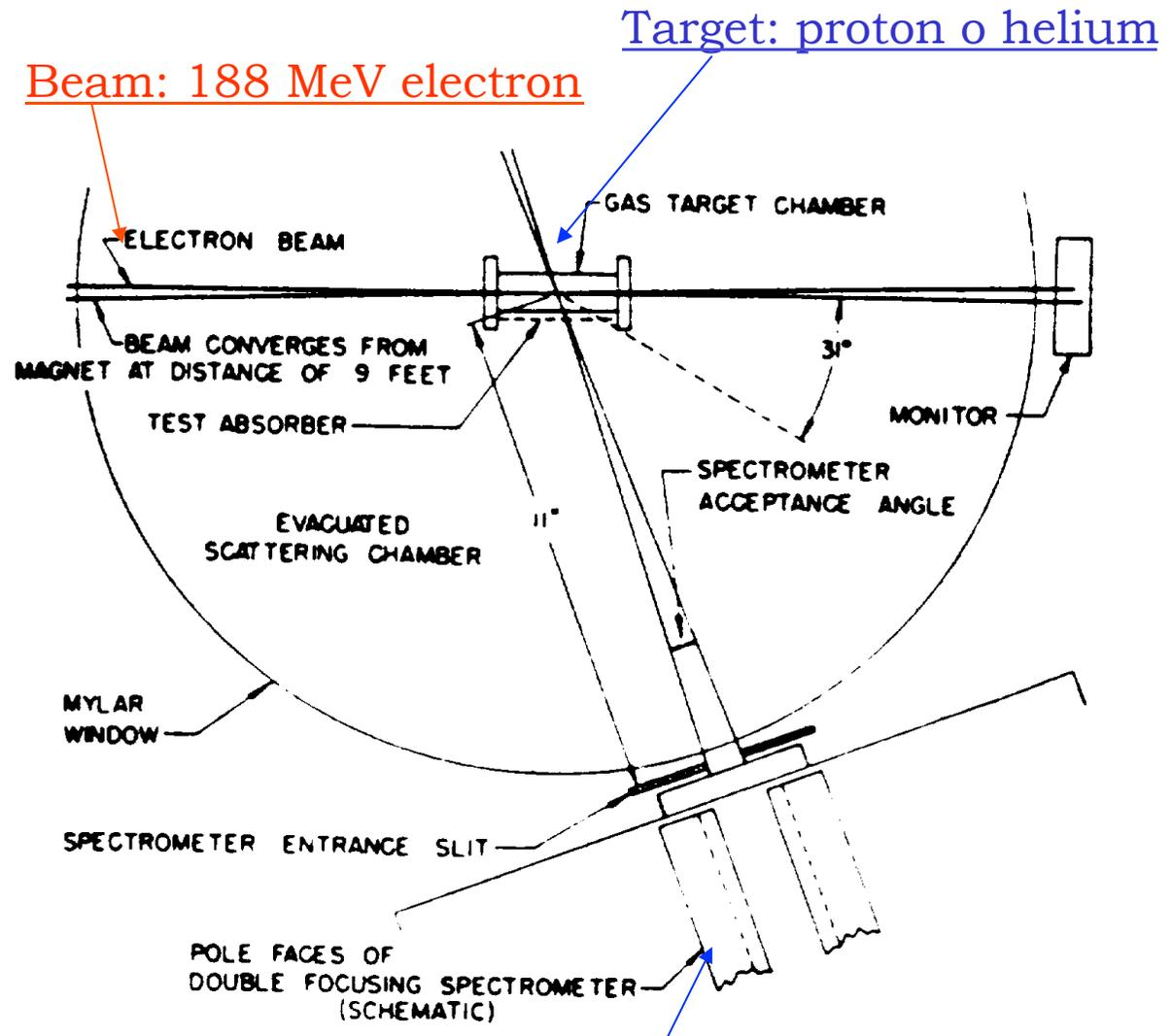
Spectrometer to measure the scattering angle. The angle  $\theta$  range from  $35^\circ$  to  $138^\circ$
