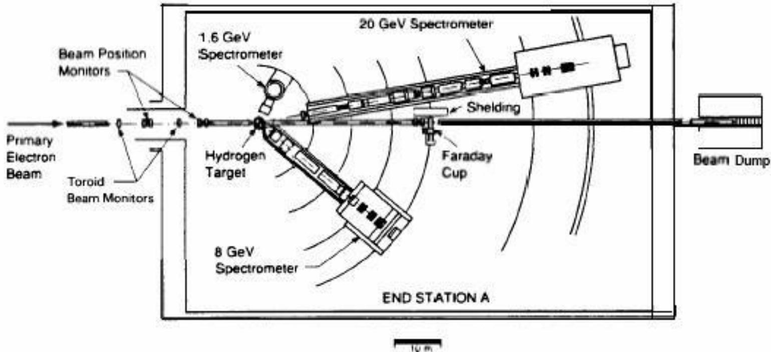
Fig. 14. Layout of spectrometers in End Station A. All three spectrometers can be rotated about the pivot. The 20 GeV spectrometer can be operated from about  $1\frac{1}{2}^\circ$  to  $25^\circ$ , the 8 GeV from about  $12^\circ$  to over  $90^\circ$ . The 1.6 GeV spectrometer coverage is from  $\sim 50^\circ - 150^\circ$ .
