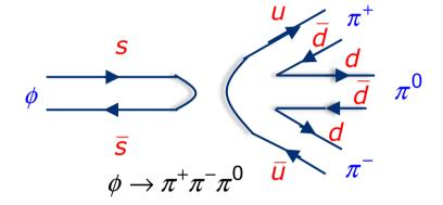
OZI rule: whenever there are quark lines not connected, the diagrams are suppressed
