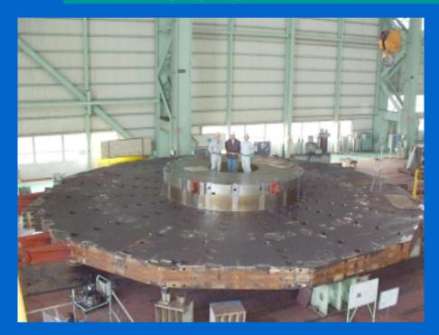
YB-2, YB-1, YB0 ready, YB1 started. Central wheel YB0, supporting the vacuum tank. Web camera !!! http://cmsdoc.cern.ch/outreach/
