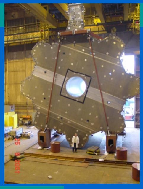
End-Cap cryostat during construction
