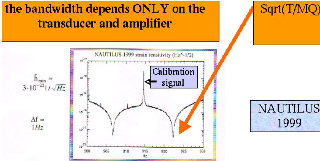
Figure 1: Nautilus strain sensitivity during the 1999 run. The x-axis is the frequency, in the range 900-930 Hz. The y-axis is in units of  $1/\sqrt{\text{Hz}}$ . The strain sensitivity at the two resonances is  $\tilde{h} = 3 \cdot 10^{-22}/\sqrt{\text{Hz}}$
