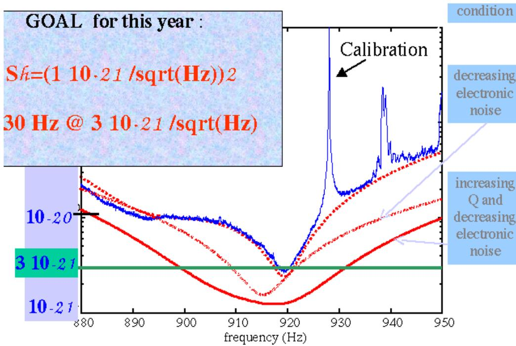
Figure 4: Explorer strain noise  $1/\sqrt{\text{Hz}}$ . The actual situation is represented in the top curve, with the calibration peak. The expectation with the actual parameters, including the extra-noise, is also represented (dotted curve). The other two curves (the first and the second curve from the bottom of the figure) represent the expectations with reduced noise and increased  $Q$ .
