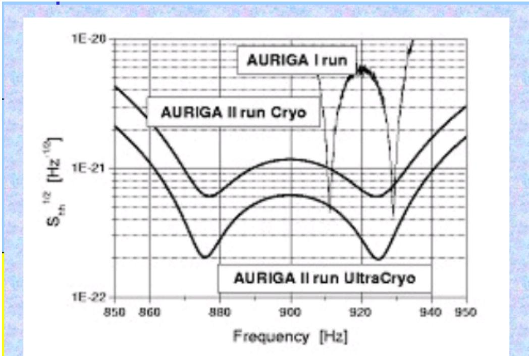
Figure 3: The Auriga expected strain noise,  $1/\sqrt{\text{Hz}}$ , with the new read-out system and suspensions. The figure shows also the strain in the 1997-1999 run: note the improvement on the bandwidth.
