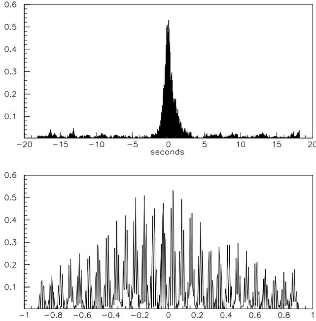
Fig. 1: The NAUTILUS response to the CR shower with particle density  $2812 \text{ par./m}^2$ , filtered energy (K) versus time (s), centered at the CR shower arrival time. The lower figure is a zoom of the upper one. We note the oscillation related to the beating of the two resonant modes and the decay due to the detector bandwidth,  $\delta f \sim 0.4 \text{ Hz}$ .
