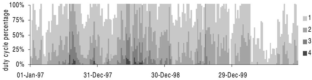
**Figure 3.** Weekly fraction of observation time for the four-fold, three-fold, two-fold and single detector configurations during 1997–2000 for an amplitude threshold of  $6 \times 10^{-21}$ /Hz from the Galactic Centre direction.
