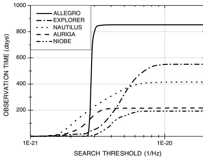
**Figure 1.** Observation time of IGEC detectors as a function of the signal search threshold for the period 1997–2000. For each detector, the ordinate is the integrated time during which the threshold set for trigger selection has been lower than the amplitude on the abscissa.
