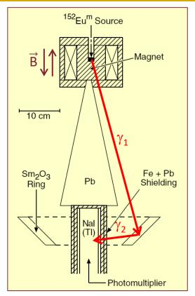
$\rightarrow$  if the excited nucleus (M) is at rest, the energy of the  $\gamma$  in the lab. is smaller than the excitation energy E<sub>0</sub>; therefore it is insufficient to excite another nucleus at rest; for this to happen, the excited nucleus has to move in the right direction with the appropriate energy.
